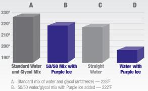
C. Straight water (no corrosion protection) — 220°F
